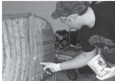
Boatbuilding Student Dan Furrow applied epoxy glue during the cold mold boat building process
